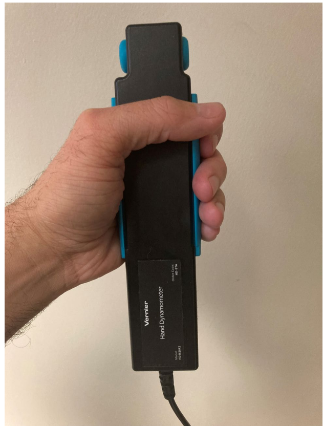
Fig. 1 Hand dynamometer. Force is applied by contracting the hand muscles, analogous to squeezing a stress ball. The dynamometer shown in this image is a Vernier HD-BTA model used by the authors in the experiments described in this paper
